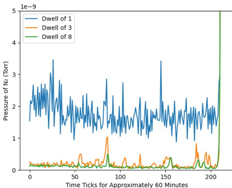
Figure 8: The Primary Mode was run for approximately 60 minutes for channels with a Dwell of 1, 3, and 8. Both the turbo pump and roughing pump were turned off at approximately the 12 minute (40th time tick) and 60 minute mark (200th time tick) respectively.
