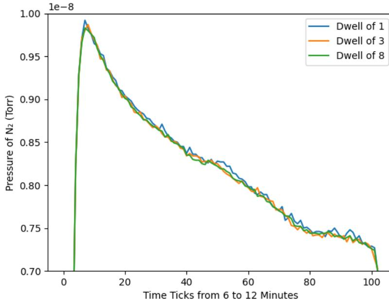
Figure 14: The zoomed in portion of Experiment 10 at its peak in pressure. Here the Dwell values of 1, 3, and 8 are compared.
