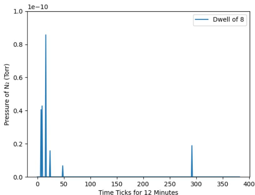
Figure 4: The Primary Mode was run for 12 minutes at a Dwell time value of 8.
