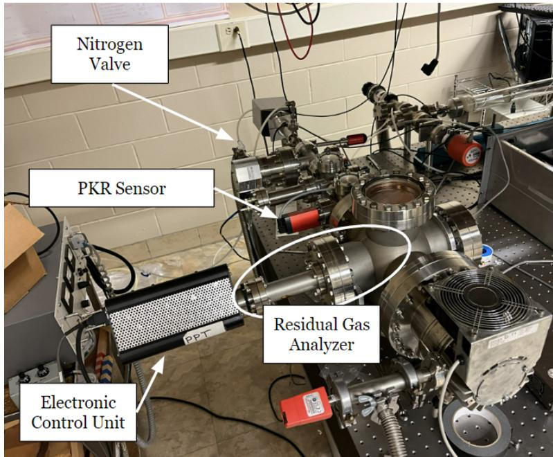
Figure 2: This is the basic experimental configuration vacuum chamber used.
