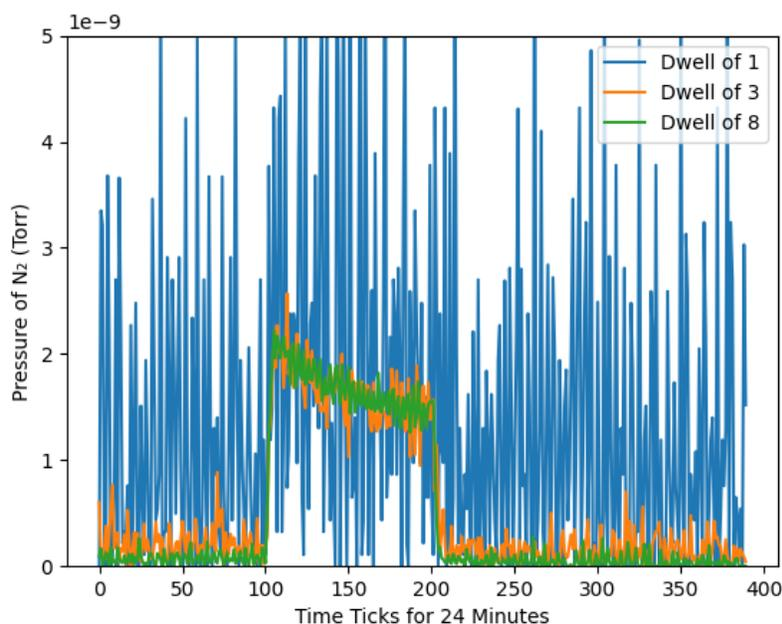
Figure 6: The Primary Mode was run for 24 minutes at Dwell times values of 1, 3, and 8. From around 100 to 200 time ticks, the  $N_2$  valve was opened to 62% and then closed.
