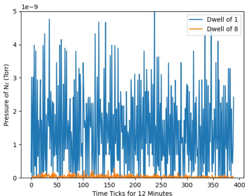
Figure 5: The Primary Mode was run for 12 minutes at Dwell time values of 1 and 8.
