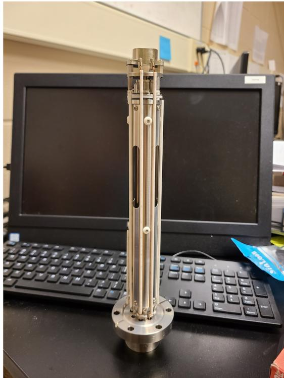
Figure 1: A picture of the residual gas analyzer (RGA) outside of the vacuum chamber.
