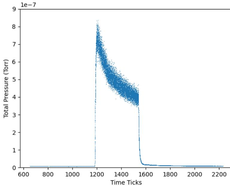
Figure 13: The PKR Full Range Gauge total pressure output over the course of Experiment 10.
