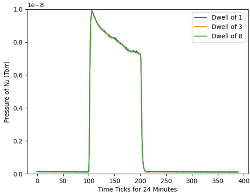
Figure 12: The SEM Mode was run for 24 minutes at 1000 volts over the channels of Dwell 1, 3, and 8. The  $N_2$  valve was opened to 62% at around 6 minutes (100th time tick) and was closed at around 12 minutes (200th time tick).
