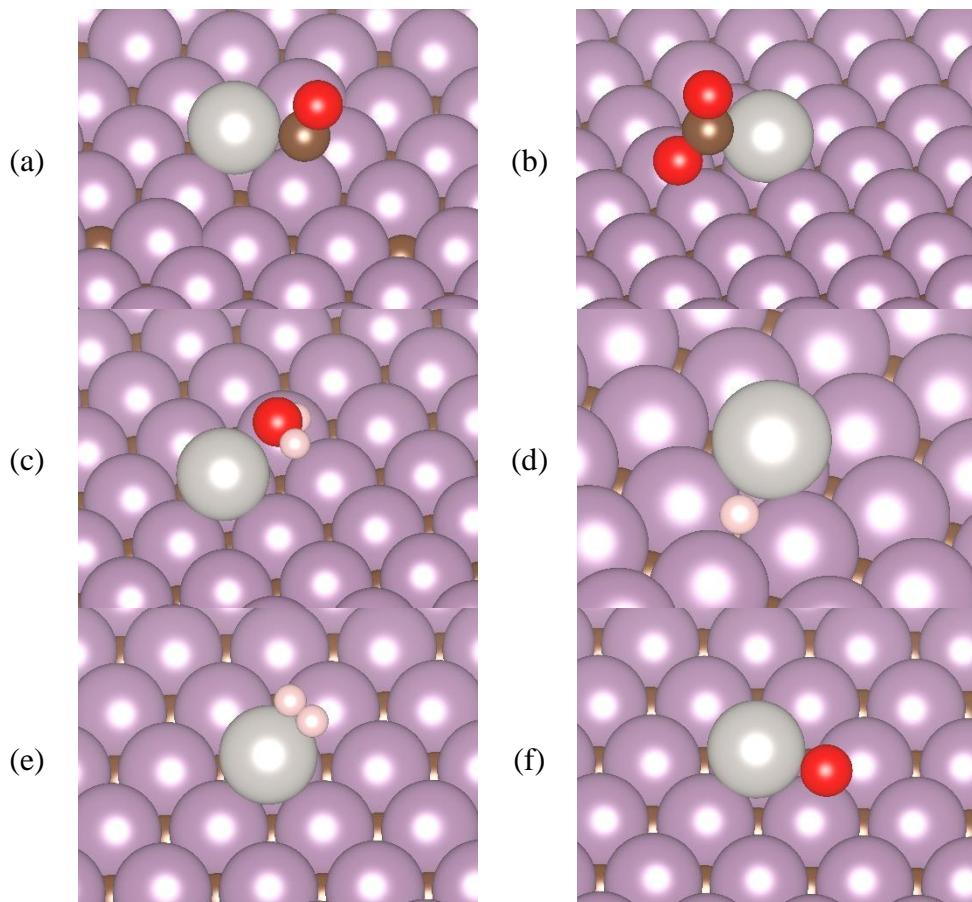
Figure 2: Lowest binding energy for (a) CO\* (b) CO<sub>2</sub>\* (c) H<sub>2</sub>O\* (d) H\* (e) H<sub>2</sub>\* (f) O\* (Mo-Purple, C-brown, Pt-silver, O-red, H-pink)
