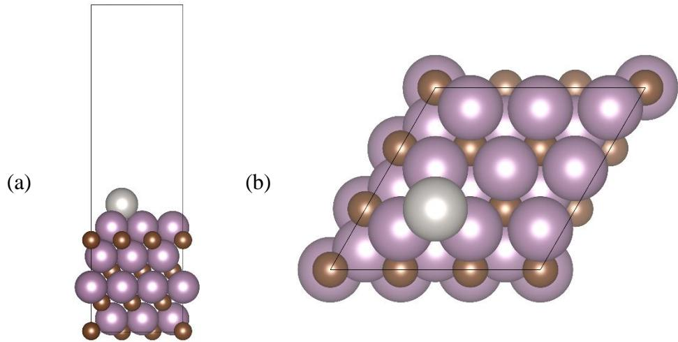
Figure 1: Supercell with single atom Platinum (a) front view (b) top view (Mo- Purple, C-brown, Pt-silver)
