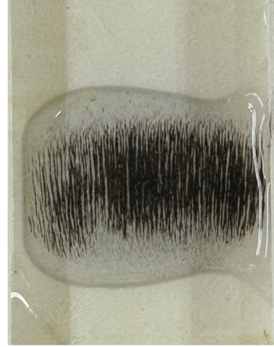
Figure 3.2: a. (top left) Micro X-ray CT scan of b-stage sheet field structured Terfenol-D magnetoelastomer coupon (0.71-micron pixel resolution). b. (top right) Cross-section view of b-stage sheet field structured Terfenol-D magnetoelastomer coupon (0.71-micron pixel resolution). c. (bottom) Sheet field structured Terfenol-D magnetoelastomer slurry coupon in a silicon mold.
