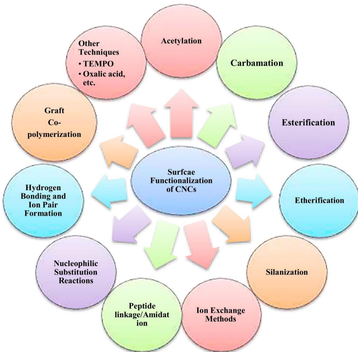
Figure 3 Surface modification of cellulose nanocrystals [33]
