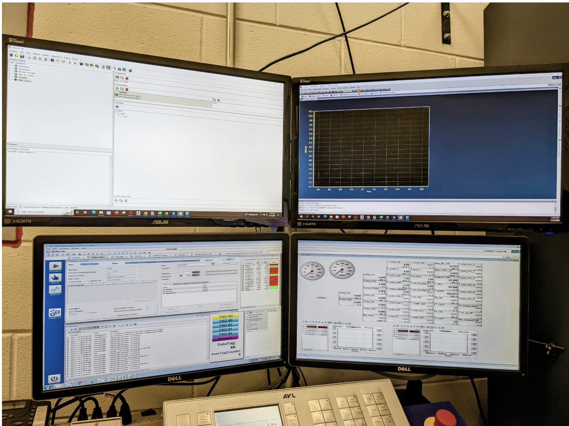
Figure 3.2: INCA, PUMA and Indicom setup for data acquisition
