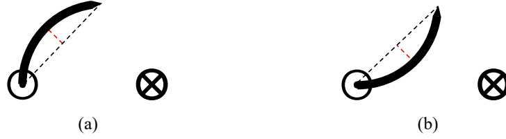
Figure 3.4: An illustration of SwayLen . (a) Positive SwayLen ; (b) Negative SwayLen . The needle, the entry point, and the exit point, SwayLen are denoted by the black curve, \odot , \otimes , and the red dashed line, respectively.
