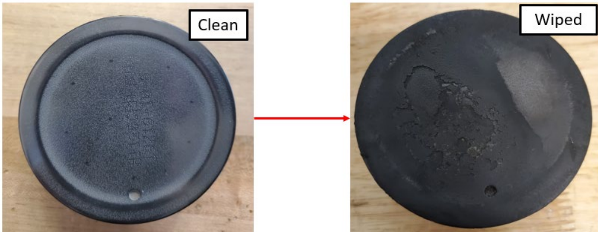
Figure 28: Coated piston before the durability test (left image) and coated piston after the durability test with CCDs forcibly removed. The exhaust side of the piston is the left side and the intake side is the right side.
