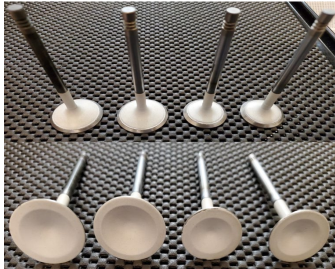
Figure 4: Gadolinium zirconate (GZO) coated combustion face, backside and stem of intake and exhaust valves
