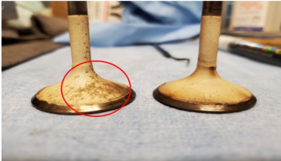
Figure 24: Fuel impingement on the backside of an intake valve (circled in red).
