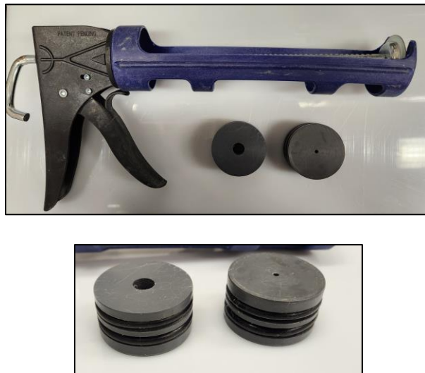
Figure 42. Caulking gun and pistons used to inject urethane resin into the outer mold. The pistons are inserted into a butyrate tube (not shown) containing resin.
