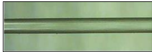
d.) Optical fiber with polyimide coating after 25 minutes of exposure to CU-7 at 120 °C.
