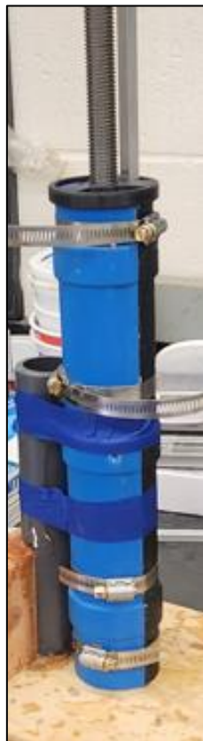
Figure 43. (a) The inner with the threaded rod in a vertical position during curing. The mold was attached to a pipe with tape. The mold was closed tight using hose clamps. (b) The inner casting has the enclosure, C-channel and threaded rod embedded in it.
