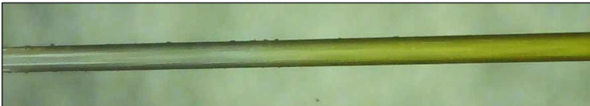
e.) Transition from intact to stripped fiber using heated Dynasolve CU-7 solvent at 120 °C.
