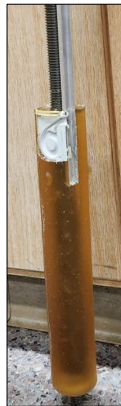
Figure 43. (a) The inner with the threaded rod in a vertical position during curing. The mold was attached to a pipe with tape. The mold was closed tight using hose clamps. (b) The inner casting has the enclosure, C-channel and threaded rod embedded in it.
