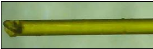
c.) Optical fiber with polyimide coating. The diameter of the fiber is 145 micron.
