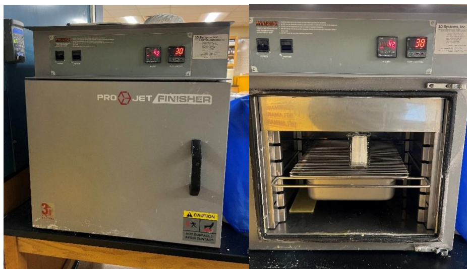
Figure 3.9. ProJet Finishing Oven used for temperature testing.
