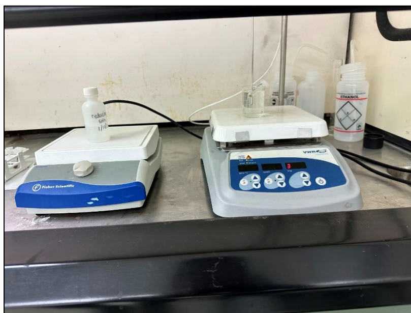
Figure 3.9: Reducing solution setup on stir plate (left) & water bath on hot plate (right)
