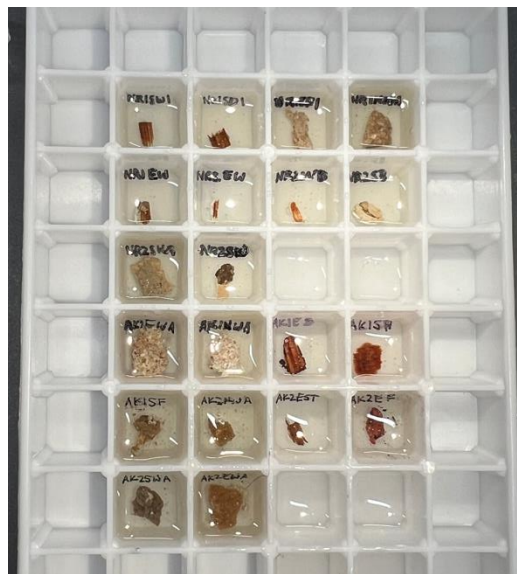
Figure 3.2 Samples from Nathaniel Russell and Aiken-Rhett house set in resin by author.
