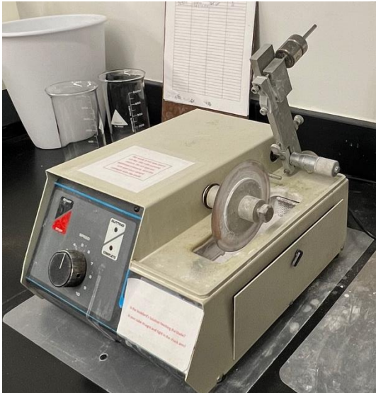
Figure 3.3 Buehler IsoMet® Low Speed Precision Cutter, image by author.
