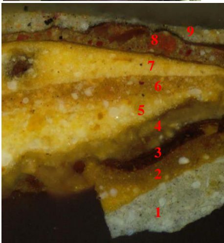
4.55 K-5. Kitchen, north wall at large hole in brick, west side Visible Light 100X
