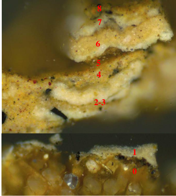
4.81 10. Detached louvered shutter, on exterior side, thick accumulations of weathered paints Visible Light 100X
