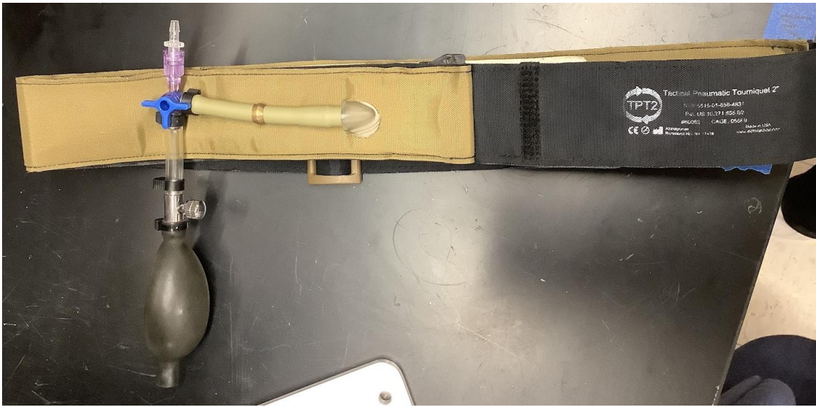
Figure 3.2. TPT2 Calibration Tourniquet with 3-Way Valve Attached
