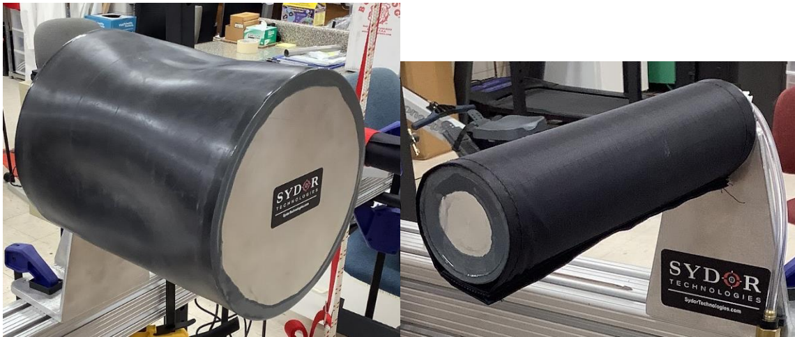
Figure 3.1. Large Test Fixture and Small Test Fixture with Nylon Sleeve
