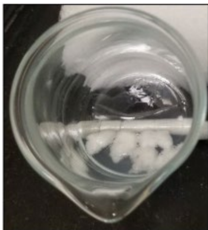
Figure 7. PLGA is dissolved in EtOH. 8
