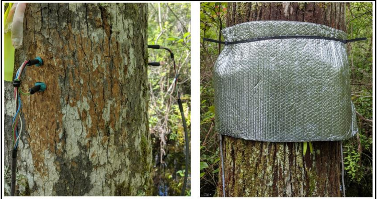
Figure 3.2. Thermal dissipation probes as deployed in the field in 2020. 4 probes were deployed at 90-degree angles around the tree, aligned with cardinal headings. Mylar shielding was used to protect the probes from rainfall and sunlight which could affect temperature readings.
