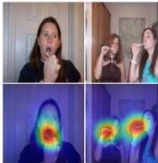
Figure 3.3 Illustration from Zhou et al. [44] showing an input image of brushing teeth and the corresponding CAM indicating the area of interest for the convolutional neural network.
