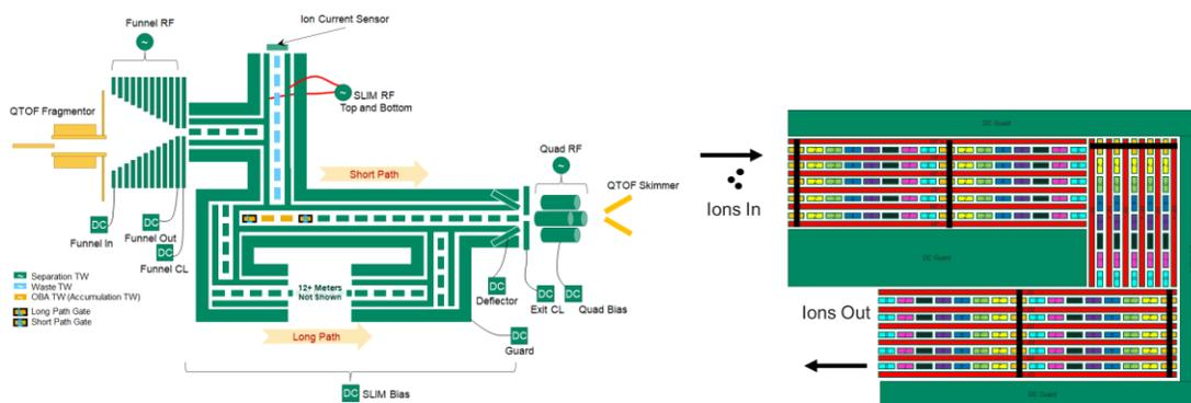
**Figure 1-9:** Schematic of the MOBILion TW-SLIM system. This instrument features a 13 m SLIM design maintained at 2.5 Torr buffer gas and approximately 25 °C.
