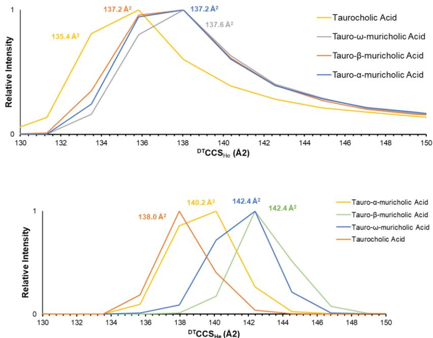
**Figure 2-3:** Graphs with different modes of data using DT helium isomeric bile acids. On top is  $[M-H]^-$  and on bottom is  $[M+Na]^+$ .
