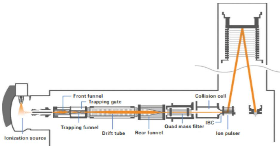
**Figure 1-8:** Schematic of the Agilent 6560 IM-QTOF instrument used. The instrument contains a 78 cm drift tube maintained at 4 Torr nitrogen at 25 °C.
